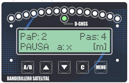
In the upper right corner of the screen "Pas" will be displayed, which will indicate the number of the pass we are currently at.
