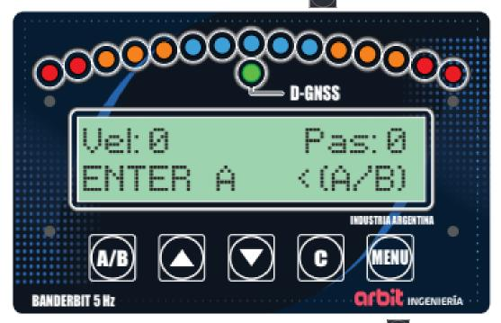
Point **B** is entered at the end of the main pass by pressing A/B again on the desired position, preferably with the machine without movement.
